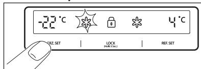
For temperature setting push **FRZ. SET** button until desired temperature displays.
