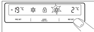
For temperature setting push **REF. SET** button until desired temperature displays.
